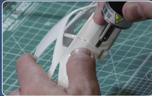
Zimmerit coating on tank model's body.
